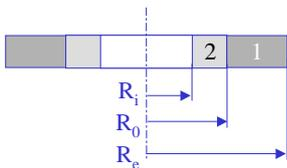
$$i = u_1 - u_2 = \frac{PR_0^3}{E_1(R_e^2 - R_0^2)} \left[ 1 - \nu + (1 + \nu) \frac{R_e^2}{R_0^2} \right] + \frac{PR_0^3}{E_2(R_0^2 - R_i^2)} \left[ 1 - \nu + (1 + \nu) \frac{R_i^2}{R_0^2} \right]$$
