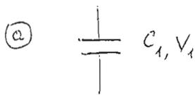
$$Q_1 = C_1 V_1 = 10^{-3} \text{ C} = 1 \text{ mC}$$
