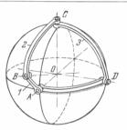
The axes of all the kinematic turning pairs should intersect at the common point O. When crank I is rotated 360° about axis OA, rocker arm 3 is turned through a certain angle  $\alpha$  about axis OD. The magnitude of angle  $\alpha$  is determined by the relations between the constant angles  $\angle$  AOB,  $\angle$  BOC,  $\angle$  COD and  $\angle$  AOD.
